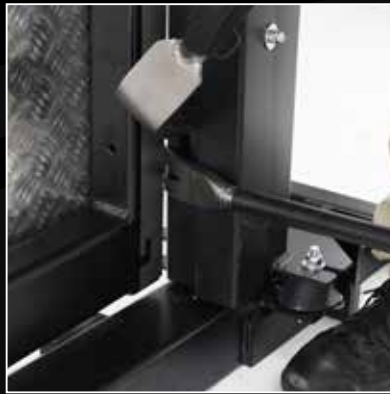
Prying in swing doors
