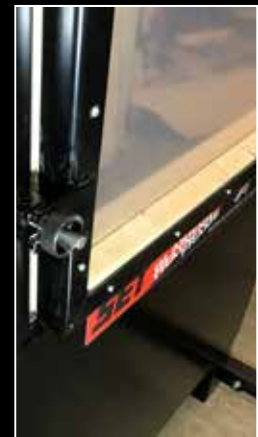
Different layers of glass or plastic sheets can be mounted to simulate various types of windows.
