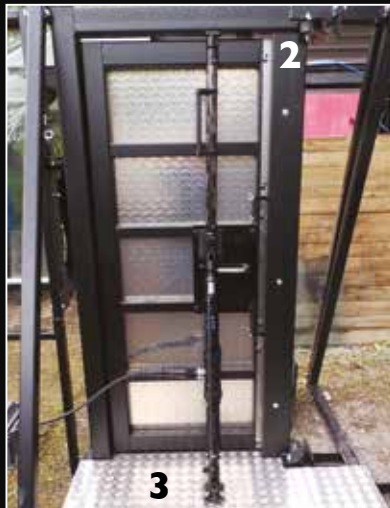
Steel pins provide the same resistance as real locks
