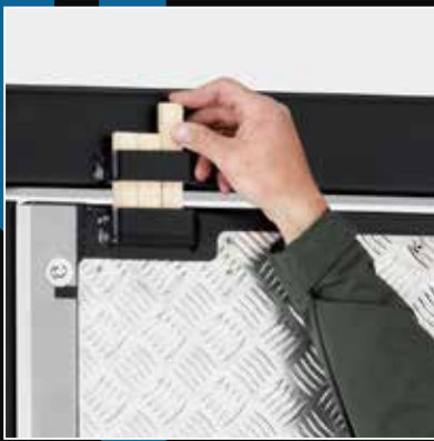
Wood Shims at top and bottom for Multi lock training
