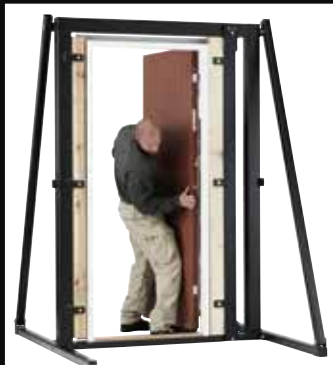
The wood frame gives a strong, realistic and easy mounting of the doors.
