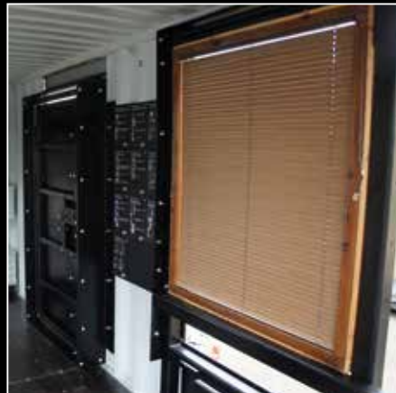
Possibility to work from in and outside and adjustable height of the window.
