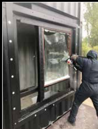
All type of breaching methods can be used on the window mounting frame.
